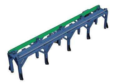
In the example above, the fixed side has been highlighted in green. all frame connectors that attach the fixed side to the frame must be tightened.
