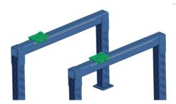
8. Place the long 45x90 extrusion you used in Step 3 on top of the gantry plates. Place the precise (machinist) level on top of the tool. If it is not level, use the leveling fixture (<u>ST-SP-016-000</u>) to correct it. Check this on both ends of the assembly to adjust the heights and level them. Do not forget to loosen the column side screws of the assembly plates before using the leveling fixture.
