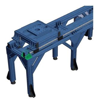
In the example above, the frame connectors and assembly plates for which all fasteners must be tightened are identified in green (one gusset and one plate).
