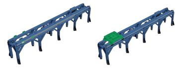
4. Move the gantry to one end of the axis and take note of any gaps or movement of the floating side. Use<u>20mm Profile Rail Shims</u> to fill gaps in the rails and <u>7/8° Slotted Shims</u> for gaps between the frame connectors to position the floating side in a stress free position. Tighten frame connectors at the location of the gantry to lock the position of the floating side in the correct location.
