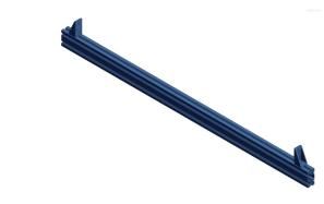
9. Place the assembled tool on top of the rails. Place the precise machinist level on top of the tool. If it is not level, use the leveling fixture <u>GT-SP-016-0001</u> to correct it. Check this on both ends of the assembly to adjust the heights and level them. Do not forget to loosen the column side screws of the assembly plates before using the leveling fixture.
