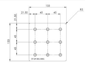
The standard Vention plate thickness is 6 mm, with the next available thickness being 11.25 mm.
