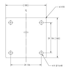
Each floor anchor has four 16.4 mm clearance holes to accommodate standard half-inch concrete anchor screws. Floor anchors also feature two layers of screws at 45 mm intervals, to maximize the number of mounting configurations.
