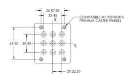
Swivel and caster wheels fit our extrusions using standard 11.25 mm thick plates. These mounting plates must have a Vention interval bolt pattern, and the bolt pattern must accommodate the swivel or caster wheel.
