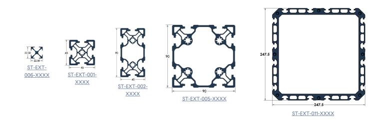
Four extrusion profiles form the core of the Vention architecture:  $22.5 \times 22.5$  mm,  $45 \times 45$  mm,  $45 \times 90$  mm,  $90 \times 90$  mm, and  $247.5 \times 247.5$  mm. These profiles are optimized for best-in-class ratios of the moment of inertia per unit of surface area.
